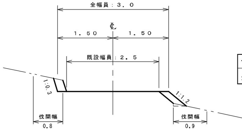
地山傾斜 =  $30^\circ$  ( $25^\circ \sim 35^\circ$ )
