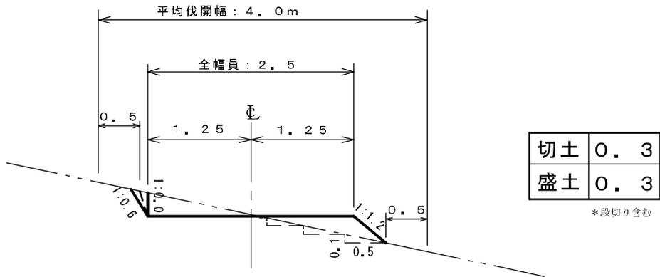
地山傾斜 =  $30^\circ$  ( $25^\circ \sim 35^\circ$ )
