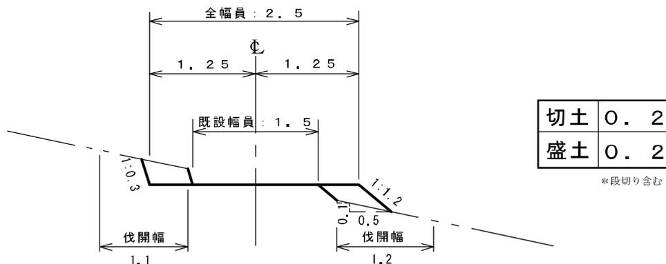
地山傾斜 =  $30^\circ$  ( $25^\circ \sim 35^\circ$ )
